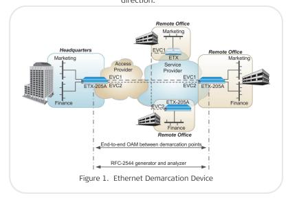
When a link failure is detected or OAM failure received, ETX-205A can shut down the affected port or forward the OAM failure message. The fault propagation mechanism enables routers and switches connected to both ends of the link to reroute the traffic to the redundancy path.
