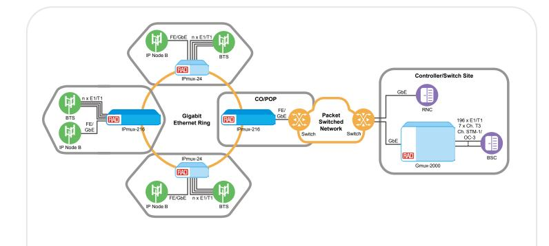
Figure 3. Delivering Ethernet and TDM Services over Fiber Ring in the First Mile
